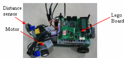
(Figure 6) Components of individual robot
