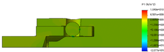
Fig. 18 The distribution of principal stress in model 3
