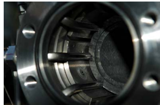
Figure 9 Cooling tubes and C/C composite inner shell test piece in the cooling structure after the heating test.
