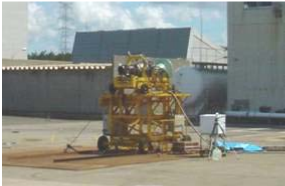
Fig. 17 turbojet engine noise test at Noshiro test center
