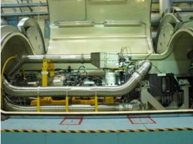
Fig. 20 JAXA ATF test of small turbojet engine
