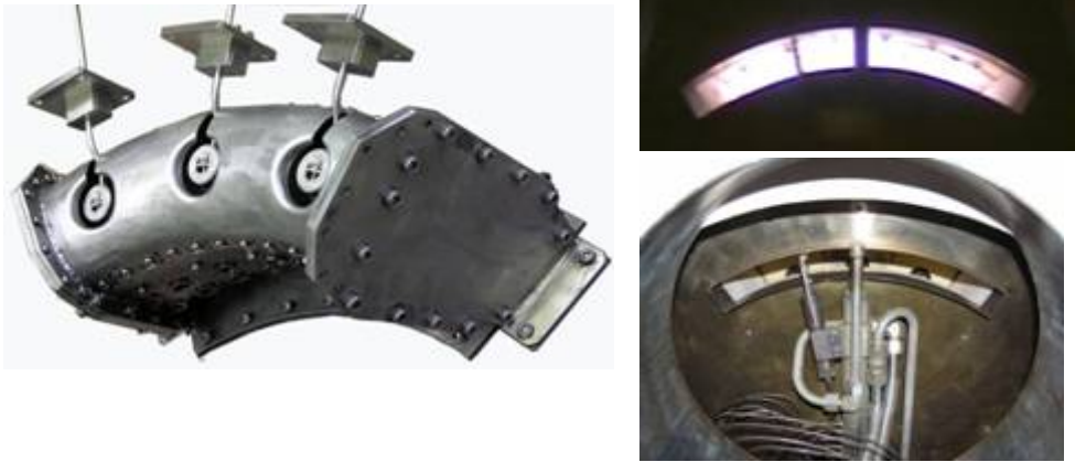
Fig. 6 Sector combustor and traverse measurement
