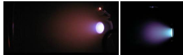
Fig. 3 Operation of the 10-mN class Hall thruster
