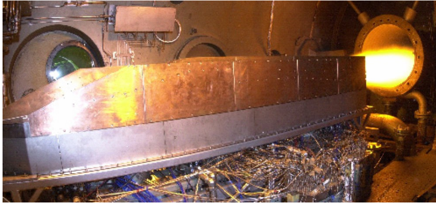
Figure 16 The engine model in the ejector-jet mode at sea-level static air condition.
