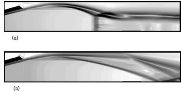
Figure 8. Shadowgraphs near shock impingement on the diffuser at motor pressure (a) 40bar and (b) 44 bar with A_d / A_t = 56.25 .
