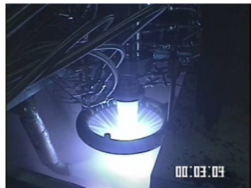
Figure 4 LOX/Ethanol hot firing test
