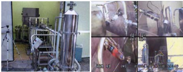
Fig. 3 Catalyst Life Test at Atmospheric Condition
