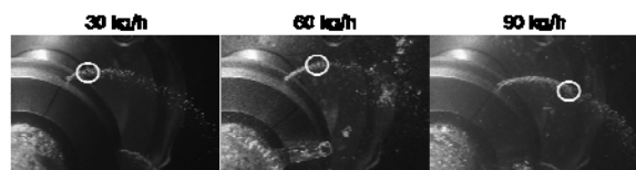
Fig. 5 Spray Visualization with Mass Flow Rate
