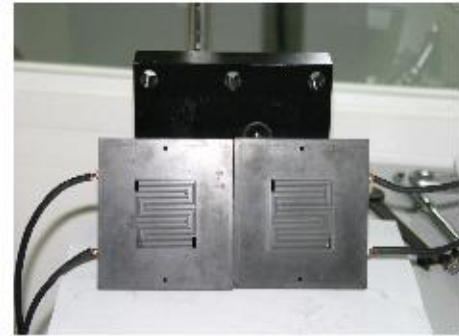
Fig. 3 Flow plates of PEMFC.
