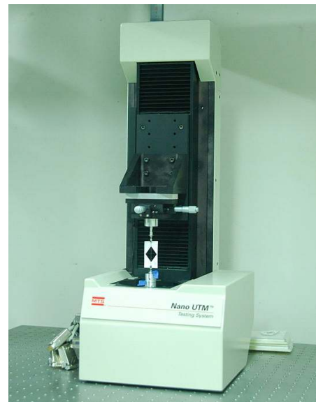
Fig. 2. Photograph of the tensile testing machine with the tensile fixture and the paper jig.
