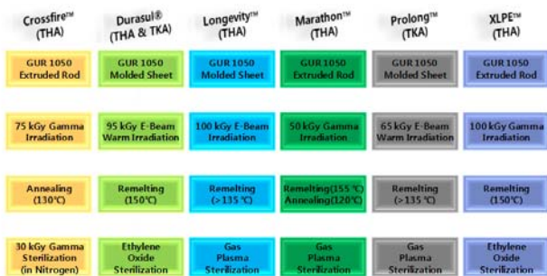
Fig. 2 Comparison of starting stock materials and processing conditions used to produce contemporary thermally treated and highly crosslinked UHMWPE materials for TKA and THA[1]
