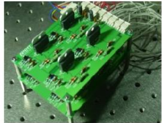
Fig.4 Amplifier developed by driving IPMC
