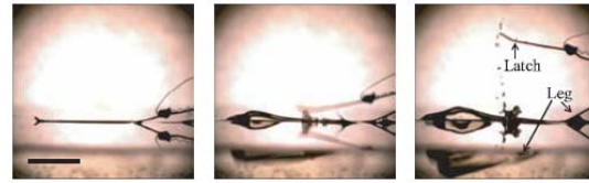
Fig. 4 Close-up view of the driving leg being released from the latch and pushing the water surface. Scale bar, 5 mm.
