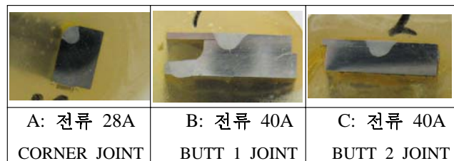
Fig. 3 Macro-sections of STS 316L endcap welds with dual rod specimens.
