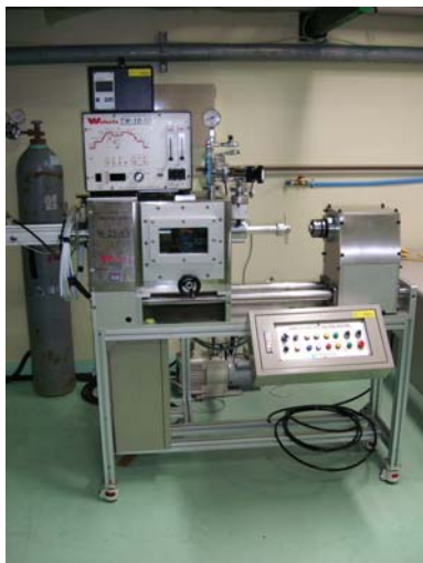
Fig. 2 Photography of the GTA welding chamber.
