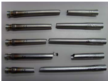
Fig. 5 Photographs of fractured tensile specimen using upper butt welding.
