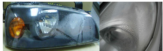
Fig. 2 Water condensing failure samples
