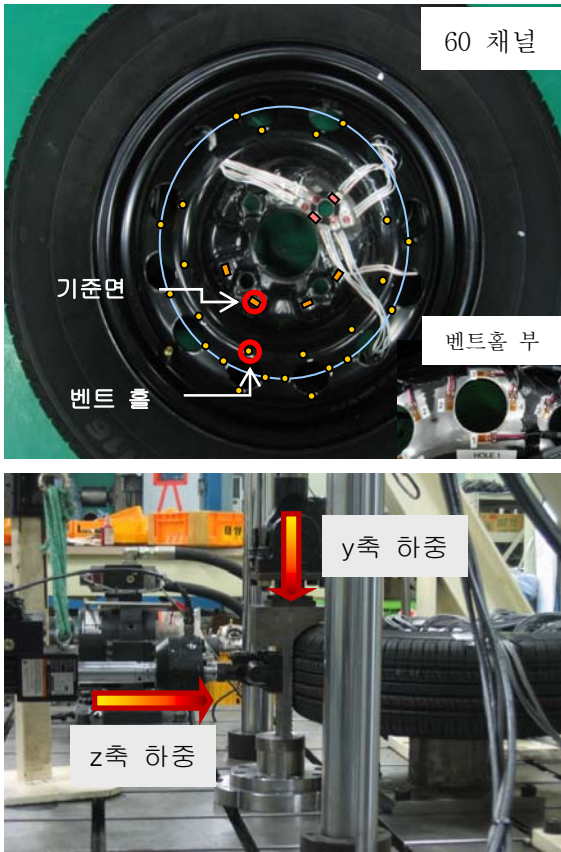
Fig.4 Stress Distribution Test on Steel Wheel
