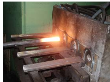
Fig. 3 Output of heating billet
