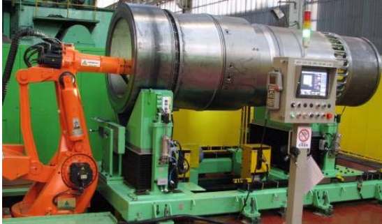
Fig. 1 Oil groove grinding robot system
