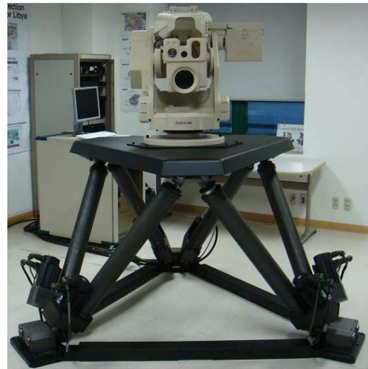
**Fig. 6** Actual system of parallel robot
