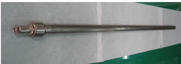
Fig 2 Photograph of seismic-resistance position indicator assembly
