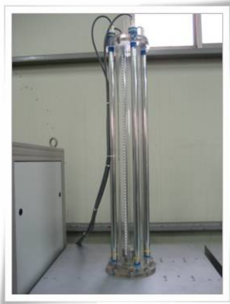
Fig. 6 Experimental apparatus of seismic-resistance position indicator
