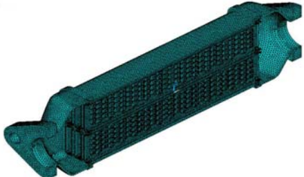
Fig. 6 Finite element model of EGR Cooler
