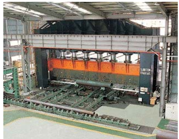
Fig. 2 Brake bending press for thick pipe forming
