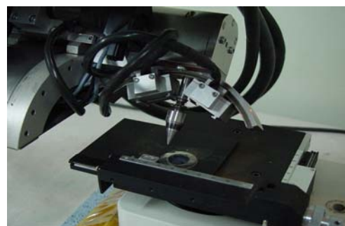
Fig. 5 Residual stress measurement by X-ray diffraction
