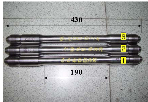
Fig. 4 Specimens for autofretting process
