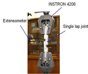
Figure 2 – Tensile-shear test of single lap joint
