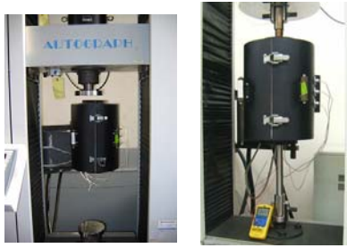
Fig. 3 Universal testing machine and furnace
