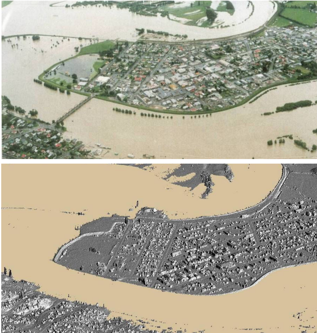
Fig. 7. Balclutha township during a 1998 flood (top) and results of 2D hydrodynamic modeling of the same flood (bottom).
