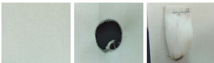
Fig. 2. Fire retardant properties of LM fabrics : (a)Untreated (b) 45° 점화법 (c) 접염법.
