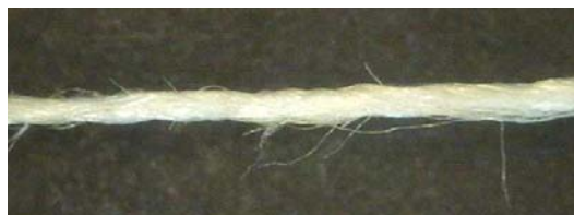
Fig. 1. Photograph of cotton like yarn(110d/180f DTY).
