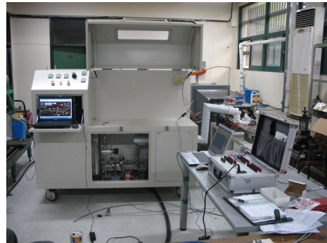
Fig. 6 Performance Test of Heat Exchanger
