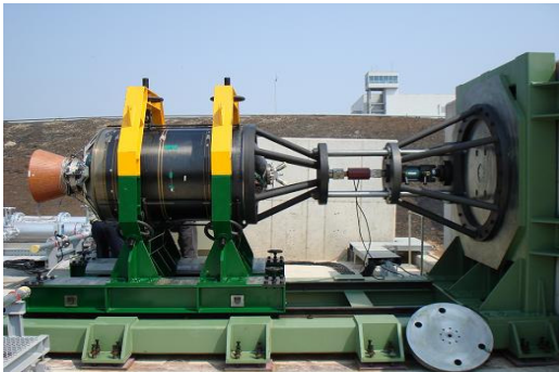
Fig. 1 Thrust Measurement System
