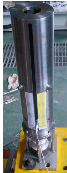
Fig. 3. Facilities of dynamic separation test in ball type bolt
