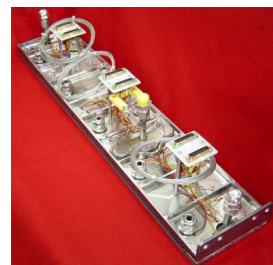
Fig. 9 Fully instrumented CMC panel before testing
