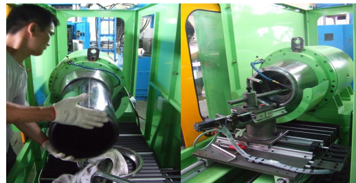
Fig. 6 Cutting Process of Rear Insulator Tube
