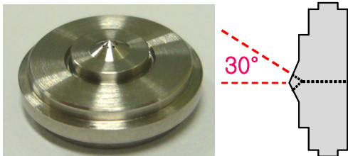
Fig. 1 Configuration of the Injector used in the Experiment
