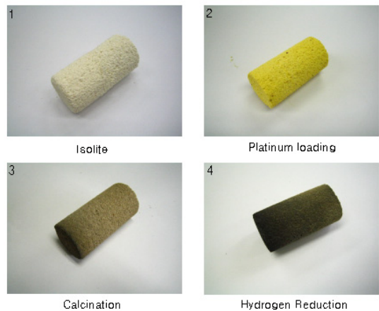
Fig. 1 Catalyst loading process
