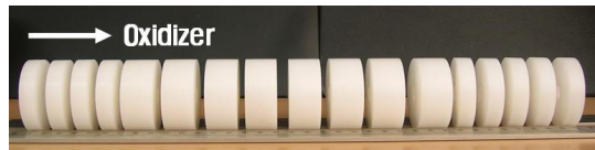
Fig. 2 Segment Solid Fuel Configuration
