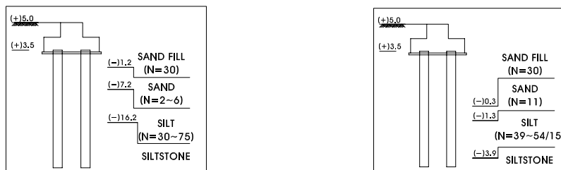
<a. 40ton Crane Foundation>
