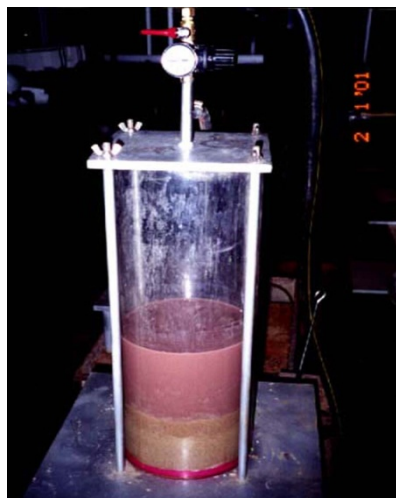
Figure. 11. The model was designed to simulate the borehole
