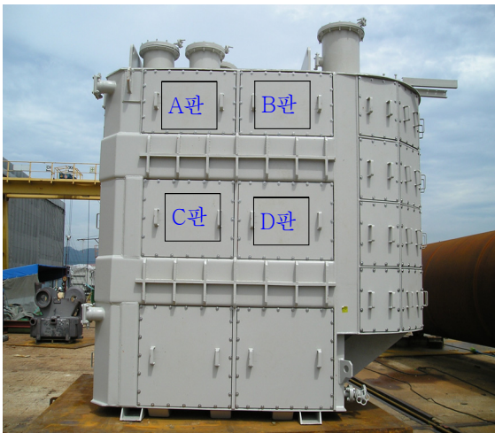
Fig. 1 Transformer for test
