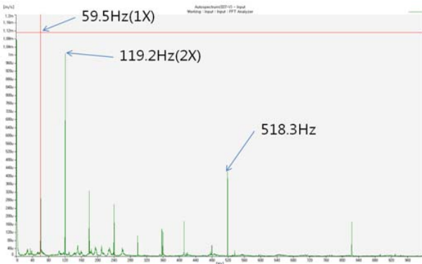
Fig. 4 The frequency spectrum in base of normal air-compressor (NDE)
