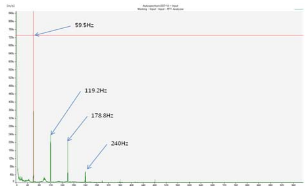
Fig. 7 Vertical direction frequency spectrum at NDE of abnormal air-compressor
