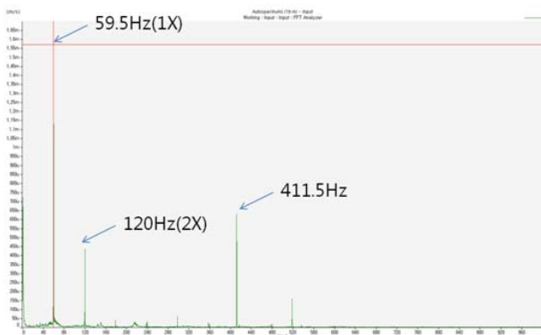
Fig. 5 The frequency spectrum in base of normal air-compressor (DE)
