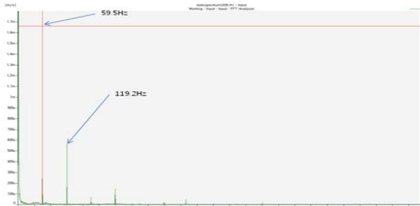
Fig. 8 Horizontal direction frequency spectrum at NDE of abnormal air-compressor
