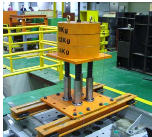
Fig. 4 The experimental set up to measure the shock-isolation using disc springs
