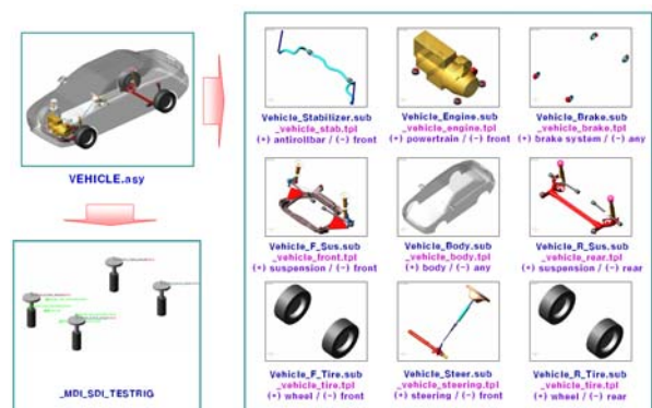
Fig. 1 Construction of the vehicle dynamics model
