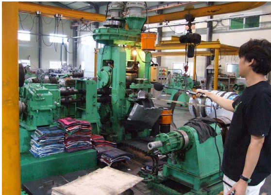
Figure 1. Measurement of the sound power level using by sound intensity probe.
