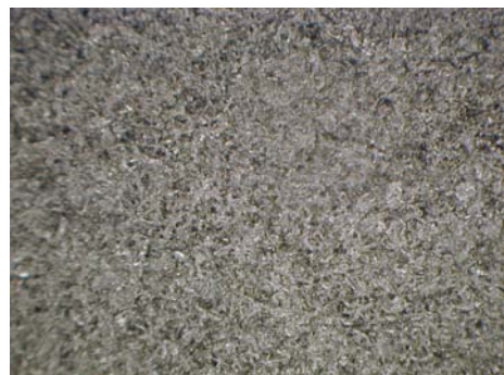
Fig. 1 Enlarged surface of porous steel absorber
