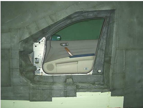
Fig. 11 Test setup of front door for two reverberant room method
