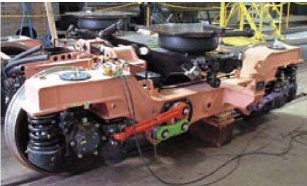
Fig. 11 Mechatronic bogie of Bombardier, Germany
