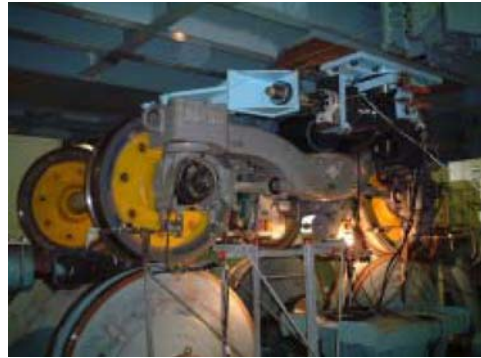
Fig. 9 Active-bogie steering truck of Japan
