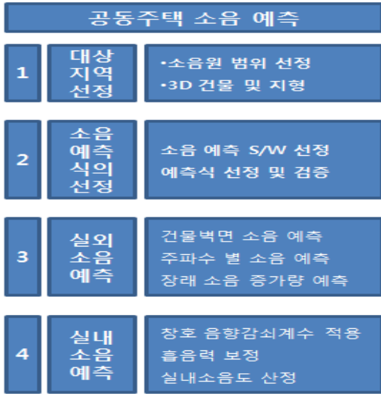
Figure 1. Procedure of sound prediction for apartment
