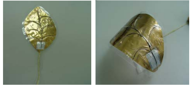
Fig. 6. An example of flower speaker made with piezoelectric Paper.
