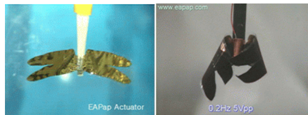
Fig. 1. Dragonfly prototype made with cellulose EAPap.
